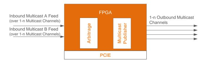
For solutions that take advantage of a hybrid hardware/software solution for message translation, the FPGA card is responsible for the following pieces of logic:
